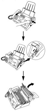
**4** Take the imaging film cartridge out of the print compartment and place it on a sheet of paper.
